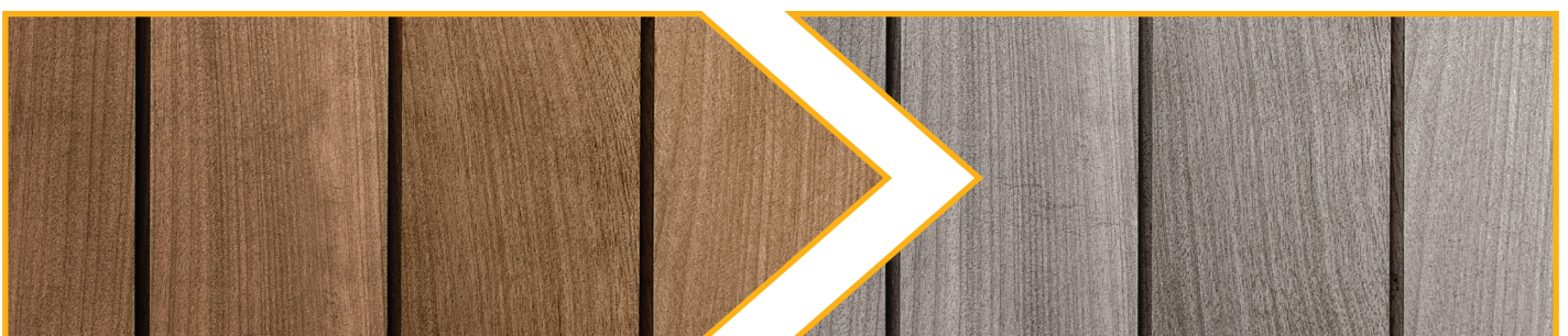
Freshly installed thermo wood before UV exposure.
