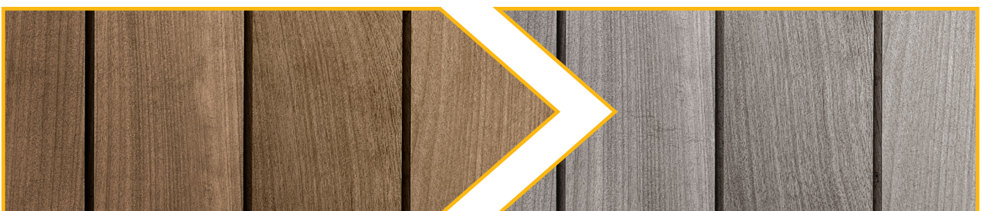
Freshly installed thermo wood before UV exposure.
